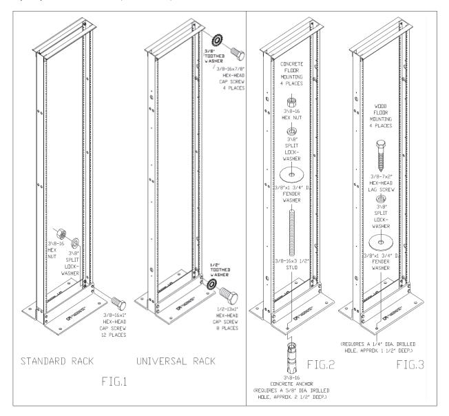
Recommended torque for #12-24 mounting screws is 30 in-lb. No particular rack maintenance is required. All CPI aluminum racks are finished with either a clear grained metal finish or powder coating finish to reduce the adverse effects of corrosion and staining.
