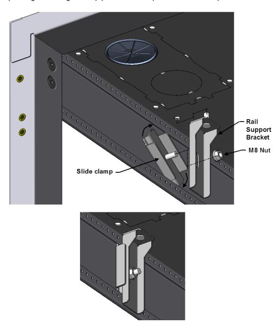
For GF-Series GlobalFrame Gen 1 Cabinets that are taller than the door frame assembly, mount the bracket assembly as shown below. Attach the top bracket to the cabinet with the M8 nut, from the Rail Support Bracket kit, onto the stud. The bottom bracket is attached to the door top rail using one of the pre-installed M6 bolts in the rail and a M6 nut and washer. Attach the bracket cover to the bottom bracket with two M4x6 screws.
