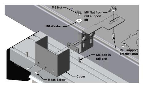
For GF-Series GlobalFrame Gen 1 Cabinets that are shorter than the door frame assembly, mount the bracket assembly as shown below; the picture is shown from the back side of the door. Attach the top bracket to the cabinet with the M8 nut, from the Rail Support Bracket kit, onto the stud. The bracket is attached to the door top rail using one of the pre-installed M6 bolts in the rail and a M6 nut and washer. The bracket cover is not needed in this type of installation.
