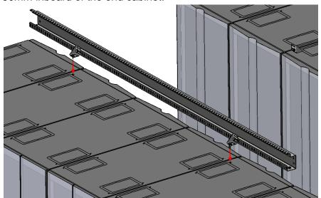
4. Loosely install gusset brackets to convenient locations along frame. Each beam length should have a minimum of two gusset bracket. Where longer beams are used, install additional brackets approximately equal distances along the length of the beams. The picture below shows the bracket installation for a GF-Series GlobalFrame Gen 1 Cabinet using M8x16 bolts, washers, and nuts.
