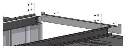
10. Install T-nuts into extrusion and loosely install lateral gusset plates on both sides of extrusion.
