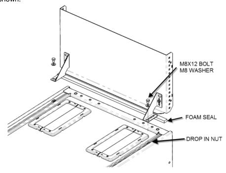
4. Locate the frame panels by aligning with the shallowest cabinet.
