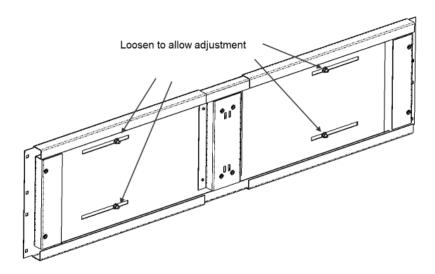
2. Install the header to the end of row duct panels using M6X16 carriage bolts and M6 flange nuts and washers. Check frame squareness and retighten the 4 M6 nuts to secure the header length.
