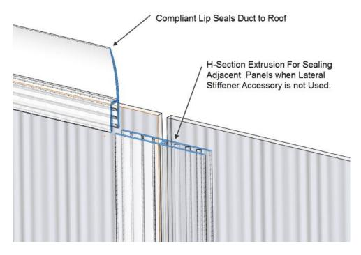
5. Install air stops between corner panel and poly panels by slotting vertical flange into upper seal
