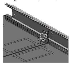
5. Attach neighboring beam sections using the provided splice brackets as shown using M8X16 bolts.
