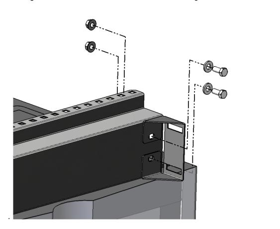
9. Attach the lateral end headers across the aisle as shown using M8 nuts and washers.
