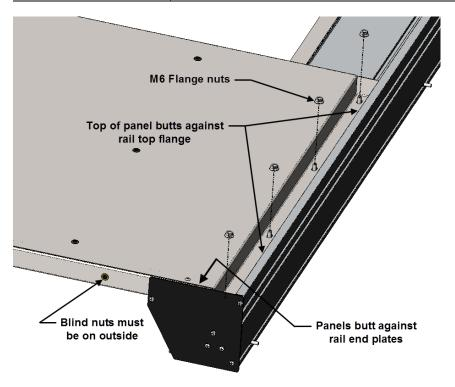
Single Door Assemblies shown below – note position of large and small panels.
