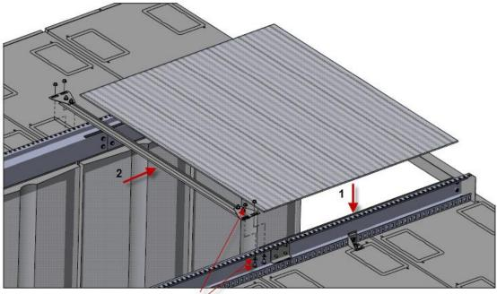
3 Fasten lateral assembly to support beams with M8X16 Screws, M8 Washers and M8 Flange Nuts
