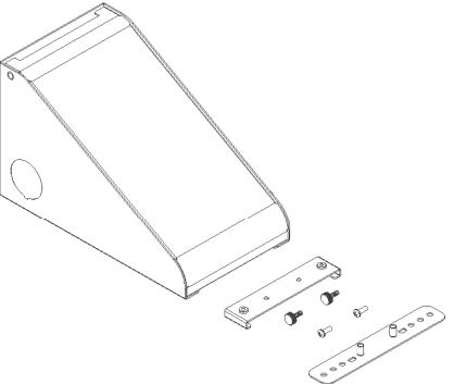
Assemble the T-Bar by installing the thumb screws from the same side as the threaded inserts. Screw the thumb screws in a few turns, leaving a space between the bottom of the screw and the tabs on the bottom side of the T-Bar.
