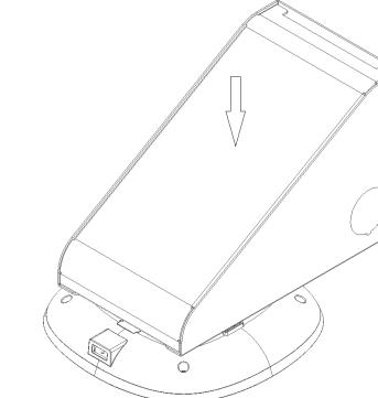
Complete the installation by placing the cover back on the base to cover the Ethernet cable and wall opening. Note that the cover can be either lifted off by lifting straight up, or the two (2) pegs the cover sit on can be used as a hinging device.
