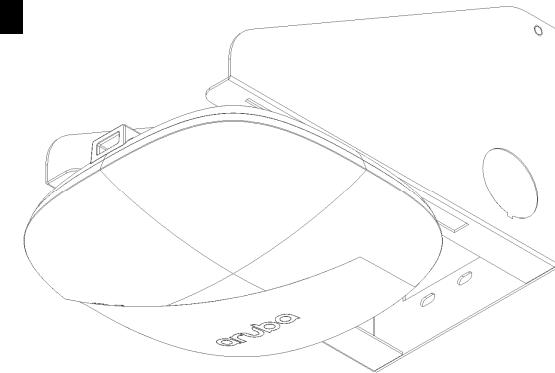
(For Aruba 3XX Series Only) – Attach the Aruba Access point to the previously installed Aruba T-Bar clip. The access point should be positioned so that the Ethernet port is facing toward the wall. Attach the Ethernet cable to the access point.
