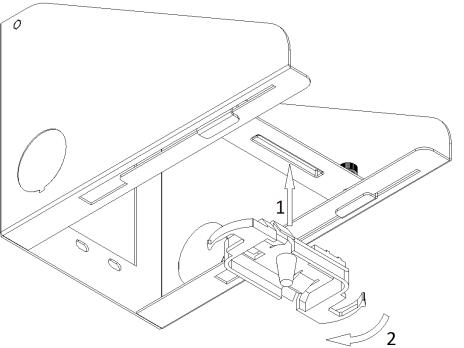
(For Aruba 3XX Series Only) – Attach the Aruba T-Bar mount to the Model 1004-00-WH T-Bar bracket by holding the Aruba mount at approximately a 45° angle and pressing it firmly onto the T-Bar then rotate the Aruba mount to lock it in position.
