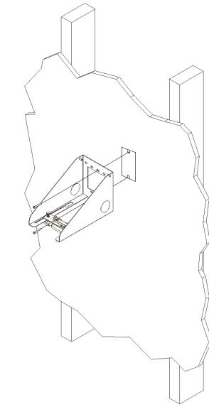
The Oberon Model 1004-00-WH right angle mount is designed to be mounted directly to either a single or double gang wall box. Use the center obround holes to attach to a single gang box and the outer sets of obround holes to mount to a double gang box.
