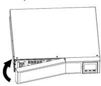
Pull out the battery box by removing two screws on the front panel.
