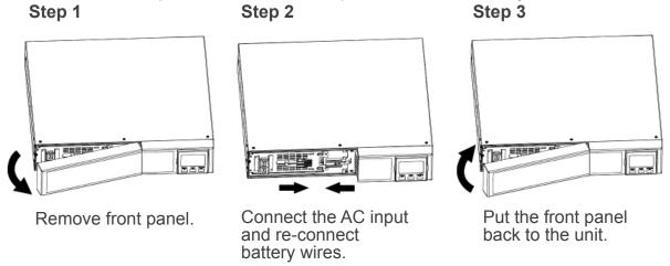
This UPS can be either displayed on the desk or mounted in the 19" rack chassis. Please choose proper installation to position this UPS
