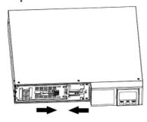
Re-connect the battery wires.
