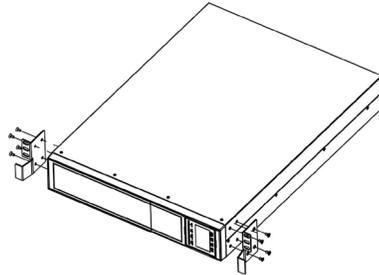
Step 2: Install the optional rack rail kits into the rack to support the UPS, Iso transformer module, and Battery Pack (one rail kit required for each piece).
