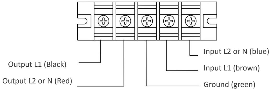
UPS Terminal Block to Anderson Connector wiring diagram
