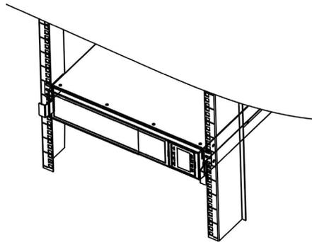
Step 4: Install the Isolation Transformer module (if included) in the rack directly below the UPS, duplicating the UPS module instructions above
