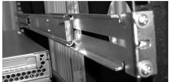
Step 3/4: Bracket, rear of cabinet
