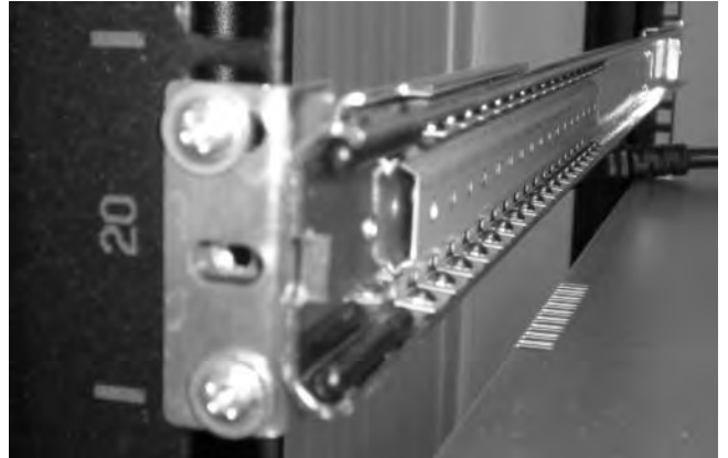
Step 3/4: Bracket, front of cabinet
