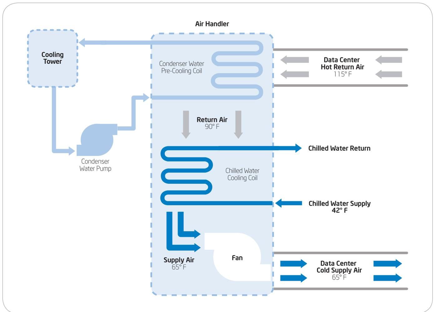
Figure 2. Decoupled wet side economizer system used with blade servers.
