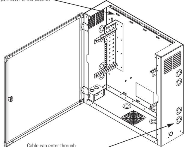
Cable can enter through knockouts or a 4" x 5" opening in back panel
