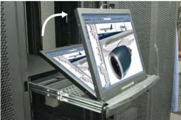
**Step 4:** Flip the front panel down and gently push the LCD display back to the rack.
