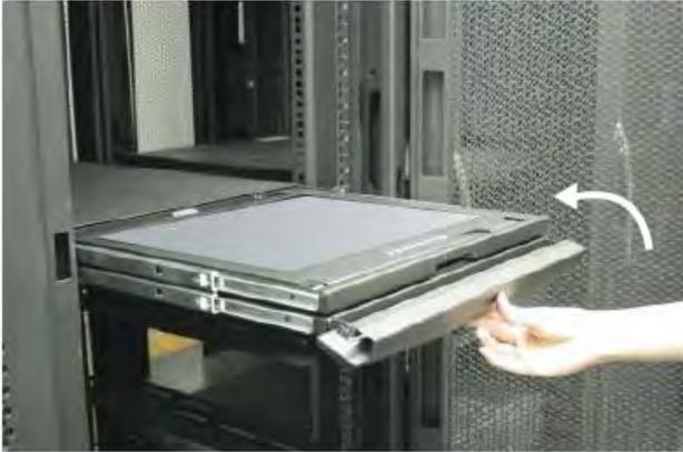
**Step 3:** Press the carry handle button and gently push the tray into the rack.
