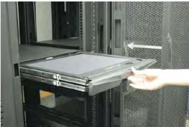
**Step 4:** When the LCD KVM Drawer is closed, release the carry handle.
