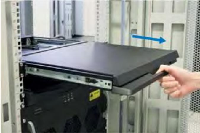
**Step 2:** When the drawer is fully extended, Flip up the LCD to a suitable viewing angle
