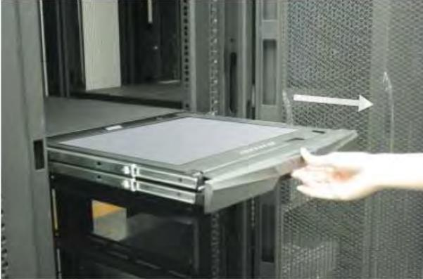
**Step 2:** When the drawer is fully extended, release the LCD panel by flipping the latch at the back of the tray.
