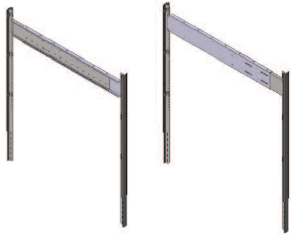
Use one Cabinet Supported Exhaust Duct Horizontal Support Beam (front and back shown) between every other cabinet along the contained aisle to connect the sides of the duct.
