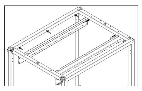
2. Lower top panel in place by sliding between screws and frame, then tighten screws.
