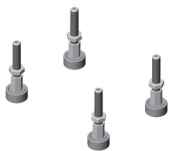
RMR Modular Enclosure Leveler Kit Leveler Kit attaches to the bottom of the enclosure if not using a plinth base. Includes four levelers with M10 threaded stems and swivel pads to help compensate for height differences in floor irregularities and jam nuts.
