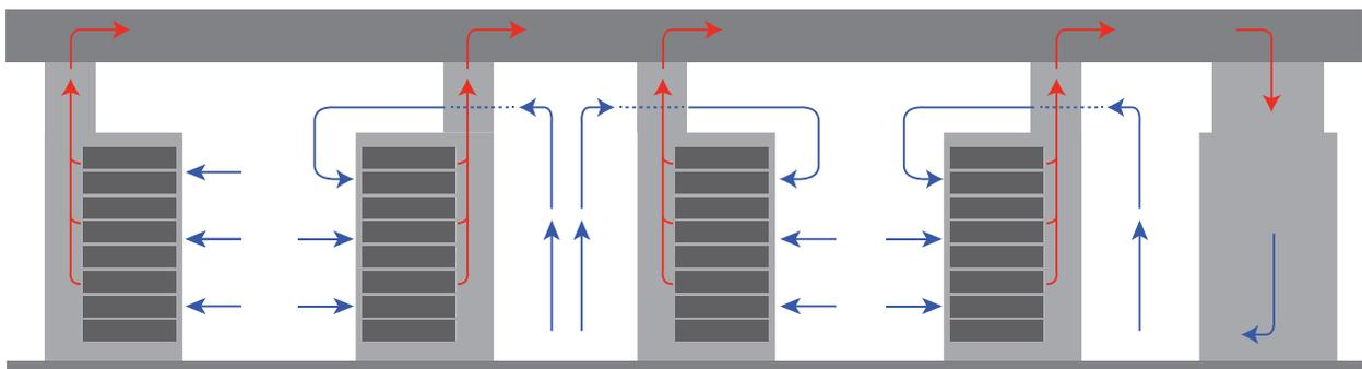
FIGURE 1: Sectional view of several ducted exhaust cabinets with Vertical Exhaust Ducts showing airflow through the cabinets and through the room.
