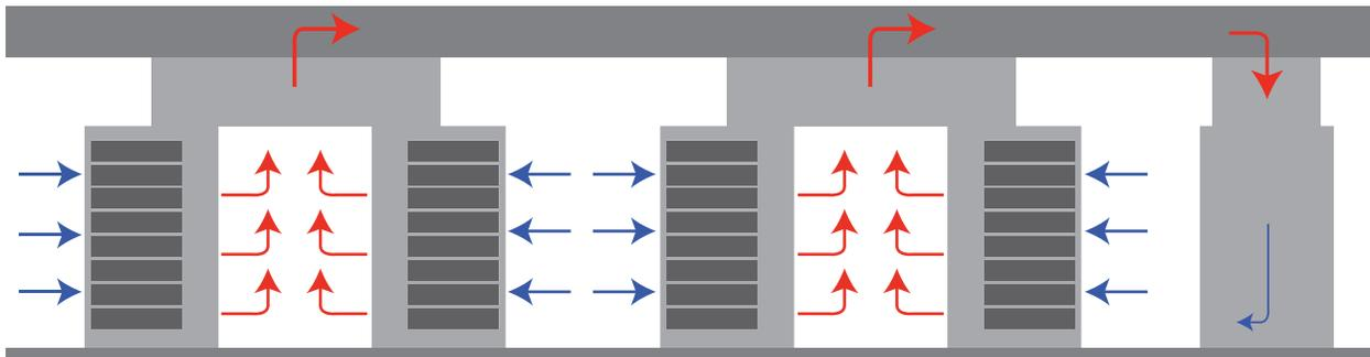
FIGURE 2: Sectional view of a HAC solution with ducts constructed over the hot aisles, showing airflow through the contained aisles and the room.
