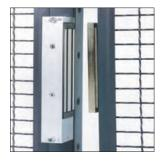
**Electronic Locks** — Electronic locking is an available option. Electronic lock mechanisms actuate on a 12-Volt or 24-Volt signal from the Building Access System (BAS). Electro-Magnetic Lock is used on sliding gates, or an Electronic Strike is used on hinged gates.
