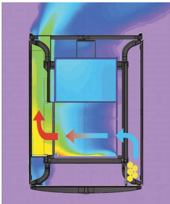
Figure 1 – Re-directing exhaust air out the rear of the cabinet
