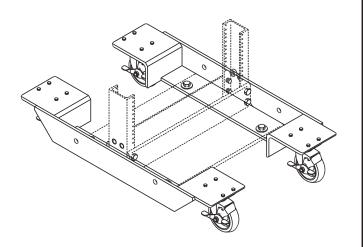
**Note:** Vertical cabling sections cannot be used on dolly-mounted racks. Can be used with 2-Post, Universal, Standard or 6' Deep Racks.
