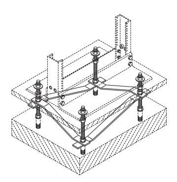
Raised Floor Rack Support includes all the hardware you need to install a CPI Standard, Universal or 6" Deep Standard Rack over a raised floor.
