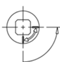
OPTION 2 FOR INSTALLATION OF ROTATION LIMITER - VIEWED FROM BACK -
