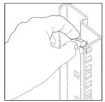
Align, squeeze, insert and release. To mount a panel, place fasteners at the same location/height/U space on opposite rails. Typically, a minimum of four Click-Nuts and screws should be used per panel. Attach panel with included screw.
