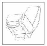
Hold Clik-Nut by the tab. Squeezing the tab allows the nut to be inserted and/or removed from mounting holes.
