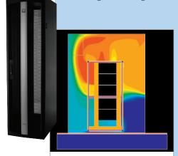
Simulation showing a typical data center server cabinet without airflow management; hot air recirculates over the top of the cabinet causing the top servers to receive air in excess of 100° (38°C)
