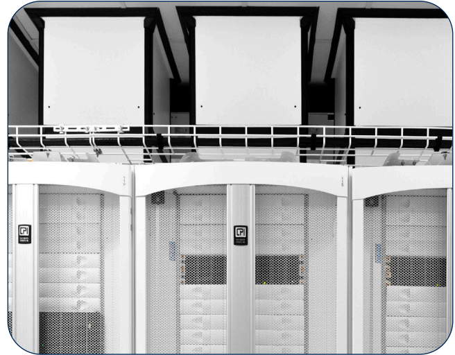
CPI’s Vertical Exhaust Ducts guide hot exhaust air from the back of the cabinet to the drop ceiling plenum, creating a closed hot air return path to the cooling system.
