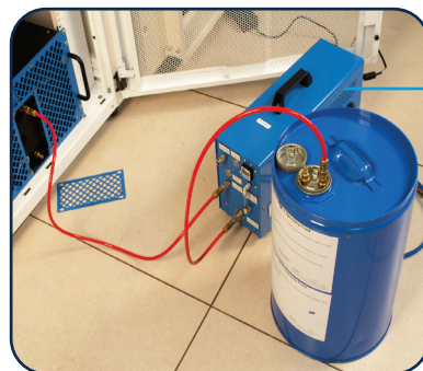
4 ZutaCore HyperCool Service Unit: Utility service unit used to pump liquid coolant into the HRU and to purge non-condensable gases out of the system
