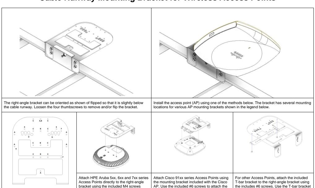
Cisco bracket to the bottom of the right-angle
