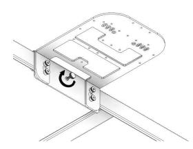
Turn the thumbscrew to secure the bracket on the cable runway. The right-angle bracket can be oriented as shown or flipped so it is slightly below the runway.
