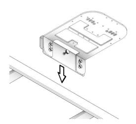
Assemble the bracket as shown and slip over the side stringer of the cable runway.
