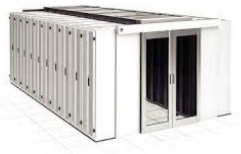
Figure 1: Cold aisle containment (CAC) directs cold air from the raised floor into the contained intake space between two cabinet rows.
