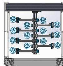
Top drawing view of Single-Sided Motive Cable Manager (P/N 32614) showing efficient use of space and smaller cable bundles.
