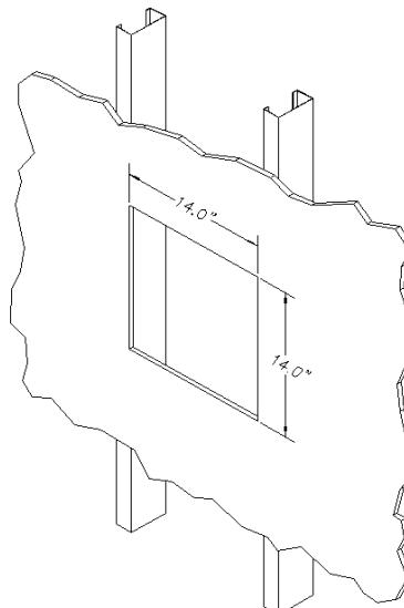
To prepare the wall/ceiling for installation, cut a 14" X 14" square hole in the gypsum board. The hole should be located centrally between two (2) adjacent studs/joists. There must be a minimum of 4" of free space available behind the wall/ceiling to allow for clearance of the enclosure.
