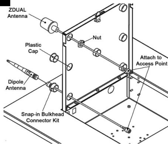
**(Optional)** If applicable, install the antenna(s) per the instructions included with optional antenna kit. After installation, connect the RF coax cable from the antenna to the access point.
