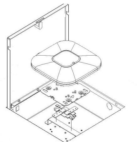
**(For Other Manufacturer's APs)** Use the manufacturer's T-bar mount clip to attach the AP to the T-bar mount. Additional components may be required from the AP manufacturer.
