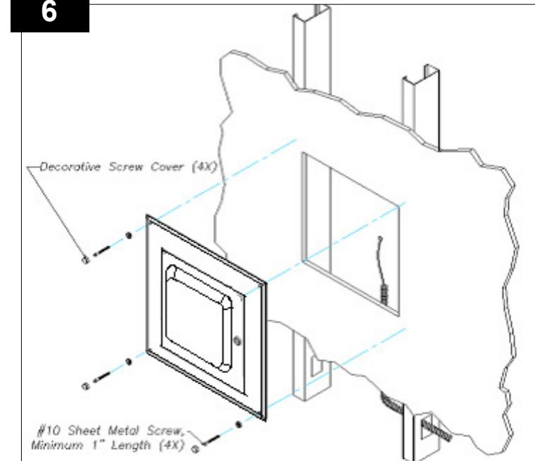
Position the enclosure so that the mounting holes are centrally located with the joists. For wood joists, use #10 wood screws (included). For metal joists, use #10 sheet metal screws (not included). The screws should be a minimum of 2" in length. To maintain pressure in pressurized rooms, use the 1051-00 and place a bead of caulking beneath the flange before installation.
