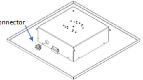
Find a flat work surface to assemble the enclosure, access point, and antenna(s) prior to mounting in the wall/ceiling.
