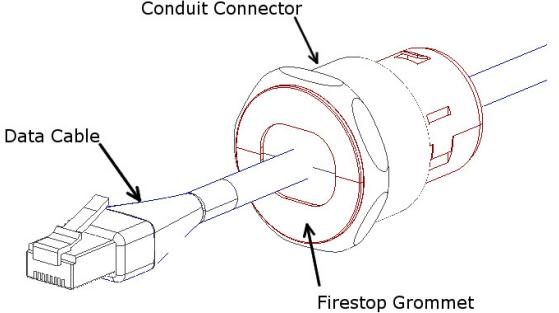
Run the data and power cable (if required) through the conduit connectors located on the sides of the enclosure assembly. Pull the data cable through the conduit connector far enough to allow attachment to the access point. Snap the firestop grommet on to the cable and slide it inside the conduit connector.
