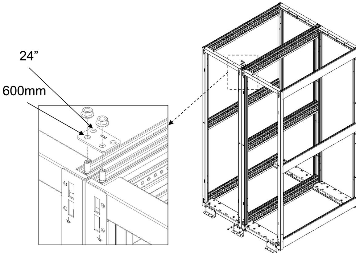
2. Move the second cabinet so that the cabinets are aligned. This may also require adjusting the leveling feet if the second cabinet was not set at the same level as the first cabinet.
