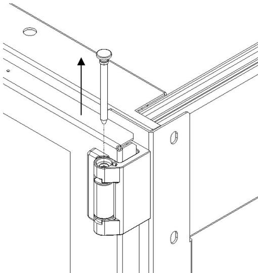
2. Open the door to exactly 90 degrees and pull the door away from the cabinet frame.
