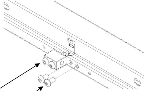
Tighten ground conductor wire binding screws to 50-55 in-lb (5.6-6.2 N-m)
