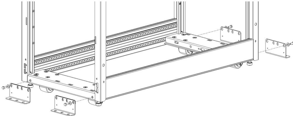
Attach the cabinet to the floor with 3/8" or M10 hardware appropriate for your type of flooring.
