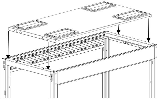
3. Pull the four (4) spring retainers until the top panel has snapped in place and secure the top panel from lifting.
