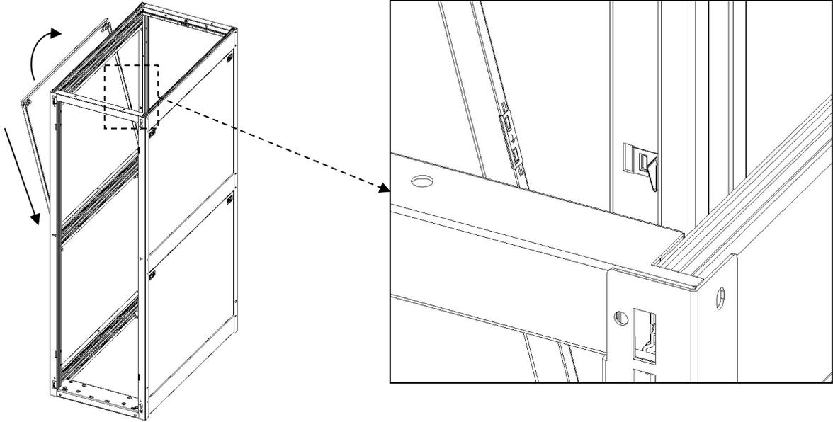
2. Rotate the side panel up to meet the frame and push until the side panel latches engage the vertical frame members next to the side panel.
