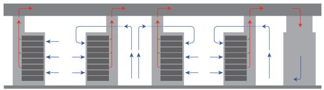
FIGURE 1: Sectional view of several ducted exhaust cabinets with Vertical Exhaust Ducts showing airflow through the cabinets and through the room. Note: Hot exhaust air is isolated and removed from the room through the Vertical Exhaust Ducts.
