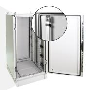
Figure 1: Openings in industrial enclosures include seals to prevent ingress of dust and liquid. Note the seal around the perimeter of the door, the channel around the door opening and the multi-point latch, which help prevent dust and liquid penetration into the enclosure. For the best protection, look for a seal that is created using formed-in-place foam gasket technology. A robotic process applies this type of seal, and it is much more durable than adhesive-backed foam tape.
