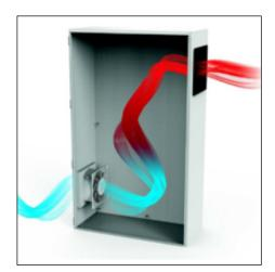
Figure 5: Recommended airflow through an industrial enclosure. Place the intake near the base and exhaust near the top. Place the filter fan on the intake to pressurize the enclosure and reduce dust penetration.
