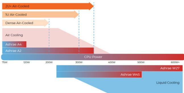
Figure 4: Transition from air cooling to liquid cooling based on CPU power and ASHRAE air-cooled and liquid-cooled classes for equipment operation. Source: ASHRAE
