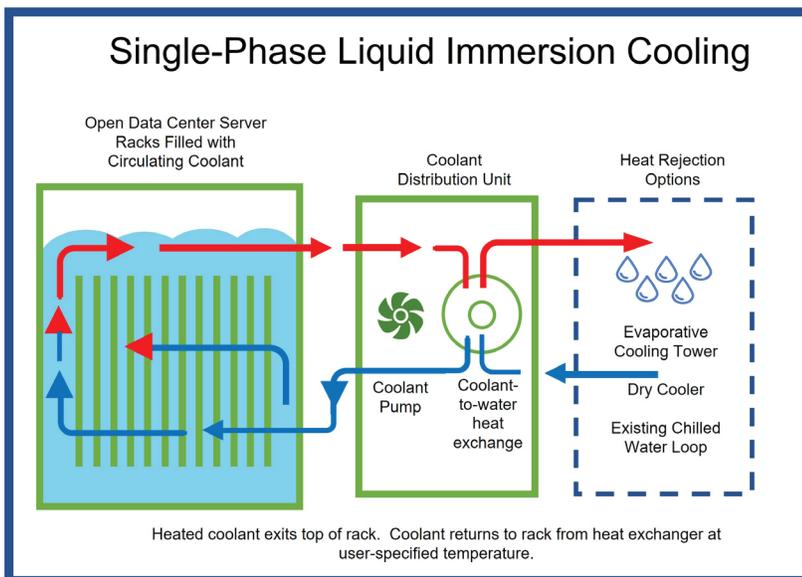
Figure 6: Single-phase liquid immersion cooling solution. Source: grcooling.com
