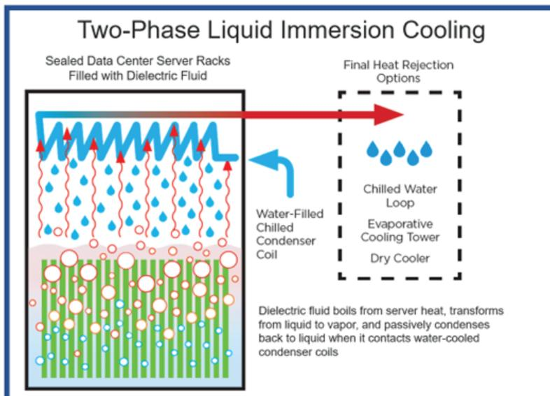
Figure 7: Two-phase liquid immersion cooling solution. Source: grcooling.com
