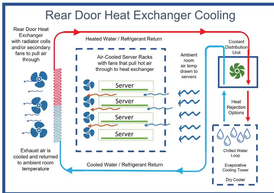
Figure 5: Rear door heat exchanger liquid cooling solution. Source: [grcooling.com](http://grcooling.com)
