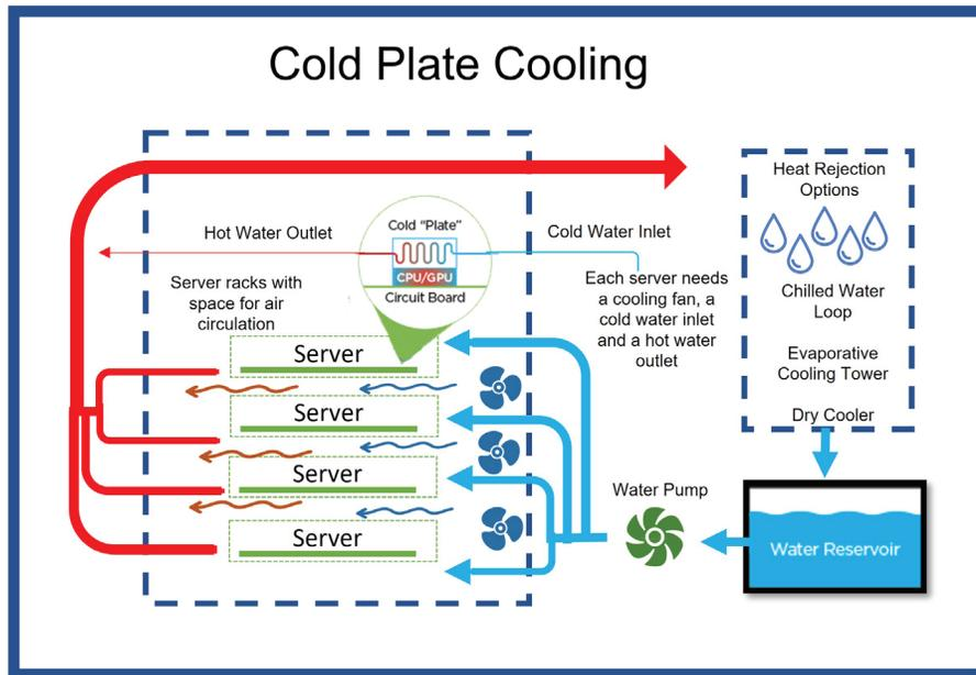
Figure 8: Direct on-chip, or cold plate, cooling solution. Source: grcooling.com
