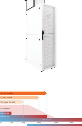
Figure 4: Transition from air cooling to liquid cooling based on CPU power and ASHRAE air-cooled and liquidcooled classes for equipment operation. Source: ASHRAE
