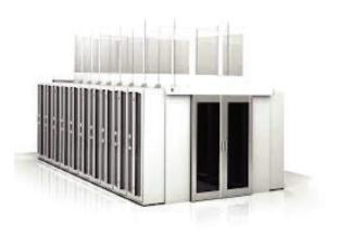
Hot aisle containment (HAC) — HAC solutions direct hot exhaust air out of the contained hot aisle to overhead return air systems. With HAC, the area outside the contained space becomes the cold aisle, resulting in a colder, more comfortable room temperature.
