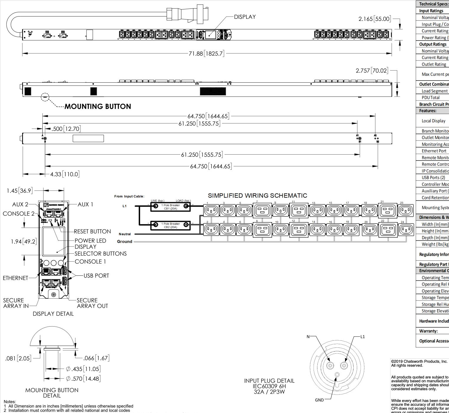
3 All Bracket kits are sold separately. Toolless mounting buttons are included for installation in CPI cabinets.
