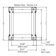
Notes: 1. There are seven depth settings for each part number as listed in the table. 2. Each rack adjusts front-to-rear in depth up to 5.91"(150 mm) in .90" (25 mm) increments. 3. Rack mounting channel depth is fixed once assembled.
