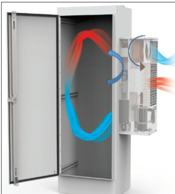
Figure 7: Cooling units provide a closed-loop system. Air is circulated within the enclosure and conditioned to a fixed set point. Heat is rejected through an air conditioning circuit to outside air.
